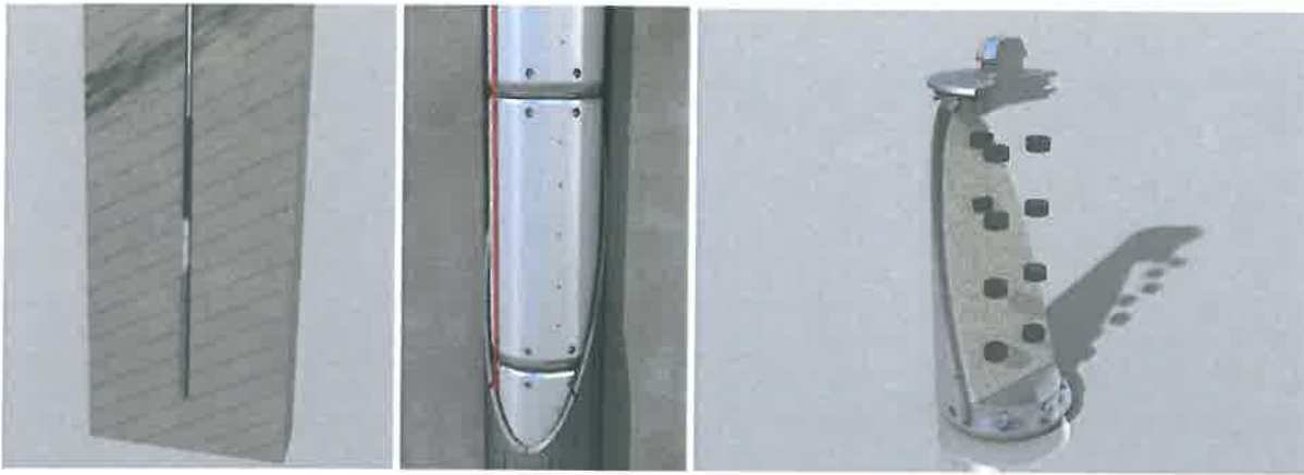
Figure 1: Borehole with modules; stainless steel module; cutaway of the module showing the distribution of steel coupons
